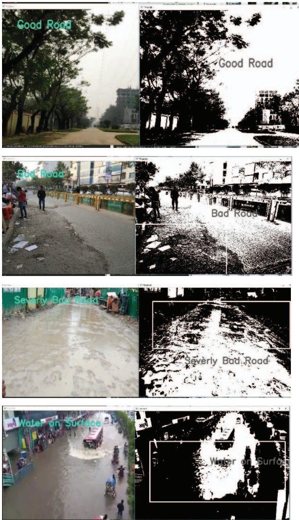
Figure 10. Test Set results of classified road and anomalies detected with image black and white thresholding
