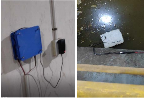
Fig. 4 (a). (Left) An STP data acquisition device in active (on power), (b) (right) An STP sensor module has been floating in the outlet pond (basement 1 of NSU)
